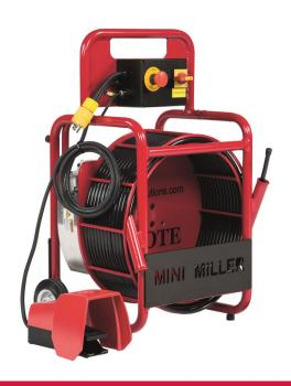
The Mini Miller is a high speed, high torque unit designed for cleaning, descaling, and removing roots in pipes between DN50-100 (2-4") pipes and for cutting/reinstatements in DN50-75 (2-3") pipe. When paired with the Picote Mini Coating Pump it is capable of brush coating in DN50-150 (2-6") pipes as well.
