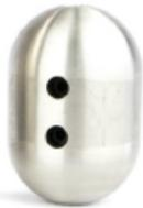
Fine-tuning tool used to pull Hub downward to remove bottom lip of the liner.
