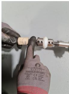
Leave a gap between the sleeve and the Smart Cutter™ Hub of approximately 6mm (1/4").
