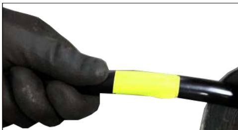
If not using a “leader” attach a visual marker (tape) on the outer casing of the flexible shaft. Place it around 500mm (20”) from the end of the shaft. The marker will indicate the tools location and help prevent possible injury from the rotating parts by alerting you when the tool is about to exit the pipe.
