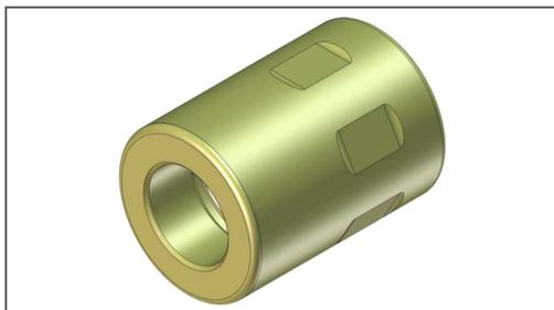
Always use a Sleeve Bearing when working with the Super Midi Miller or Super Midi Miller +C. It prolongs the lifetime of the flexible shaft and prevents the outer casing from melting in the tool end. Sleeve bearings can be reused when outer casing has been shortened.
