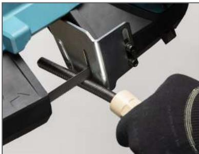
Always inspect the flexible shaft before each use. Run the machine briefly in clockwise direction to allow the shaft to return to its resting position. If there are potential weak points or the shaft is damaged, cut off the damaged length using a band saw. For most tools, the shaft should extend ~40mm (1 ½”) past the casing. Hubs and Original chains without a leader require more exposed shaft.
