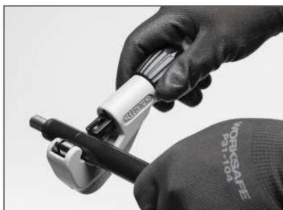
Always inspect the outer casing before each use. The easiest and safest way to shorten the outer casing to the correct length is using a sheath cutter. Only the necessary amount of bare shaft should be exposed at any time.
